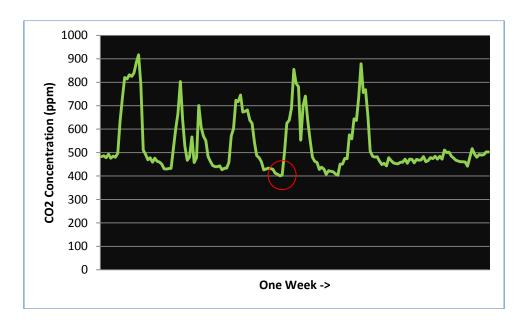
This recording from a sensor shows a typical one week recording in an office environment. The auto-calibration function uses the low point (circled) and uses it to recalibrate the zero point.
