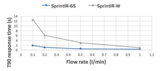
(T90 time measured from 0 to 10% CO<sub>2</sub> - digital filter switched off)
