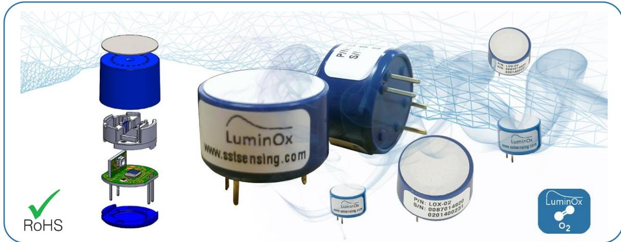
The LuminOx family (LOX) is a range of factory calibrated oxygen sensors which measure ambient oxygen partial pressure (ppO<sub>2</sub>) levels using the principle of fluorescence quenching by oxygen.
