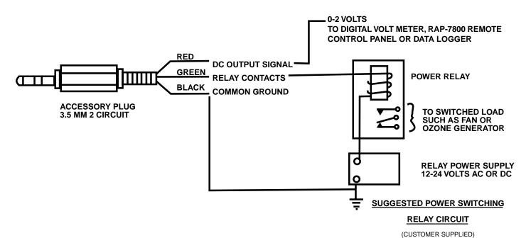
The C-21 internal relay is a "dry contact" FET device. It will handle up to 30 volts AC or DC at up to 130 ma so it will switch low voltage alarms directly. For switching power loads an intermediate relay and power supply should be used such as shown above.
