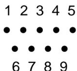
The analog voltage signal is measured across pins 1 (+) and 5 (GND). The analog current signal is measured across pins 9 (+) and 5 (GND).
